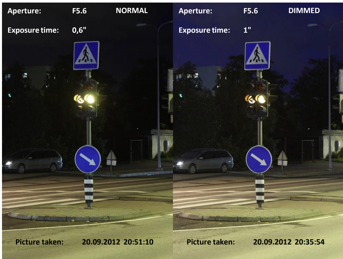
Figure 13 Difference between normal and dimmed traffic light in the scene
