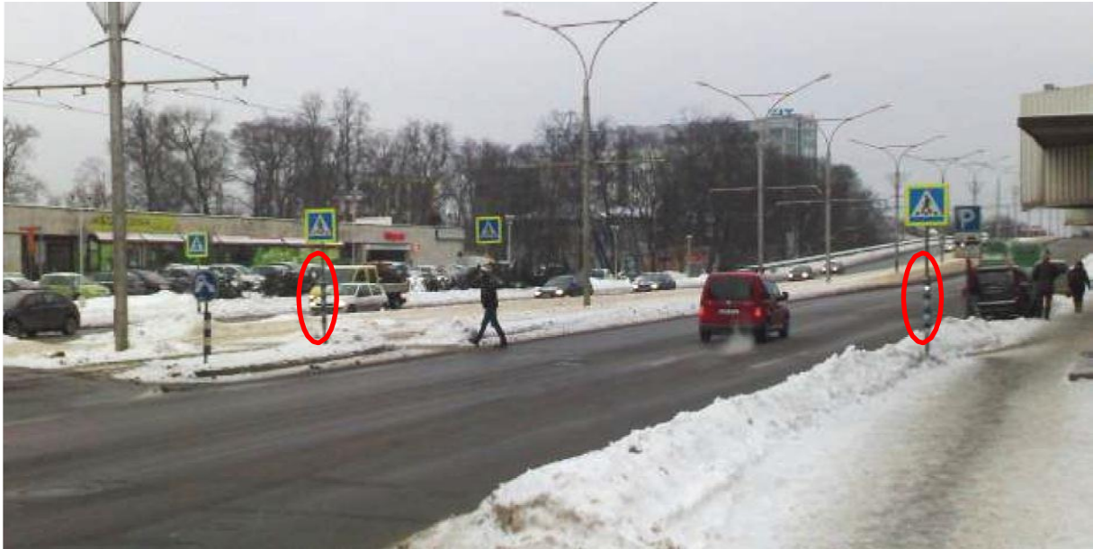
Figure 2 Pedestrian radar activated blue LED blinking reflectors on crosswalk traffic sign poles
