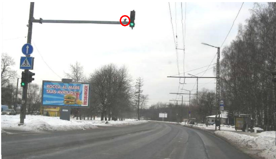
Figure 4 Traffic lights with a speed radar (sensor to the left of the upper traffic light)
