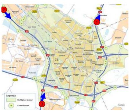
Figure C1.1.1: The three detector locations on the highways surrounding Utrecht. Each lane has its own detector (Goudappel).
