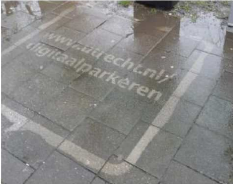
Picture B4-3: Green street graffiti: the pavement is cleaned by spraying water under high pressure on a template which showed the web page of digital parking. As a result the address of the web page shone through on the 'dirty' pavement. After about five weeks the message gradually fades.
