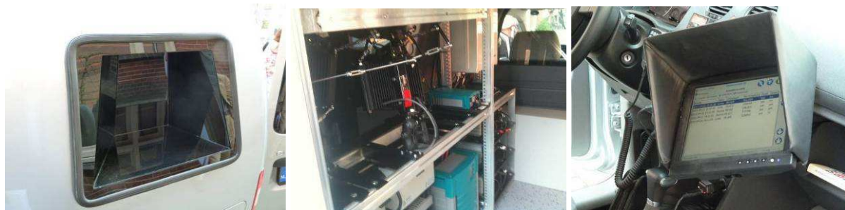
Picture B2-1: pictures of the scan-car. Left: the side of the scan car with cameras behind the mirrored glass. Middle: camera system inside the car. Right: the computer display showing information on the scanned license plates.
