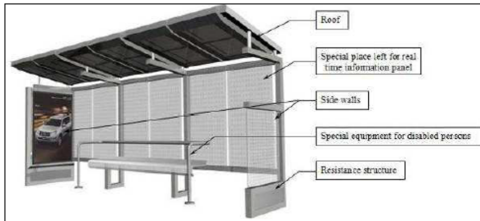
Fig. A.7 Modern bus stop shelter – structure
