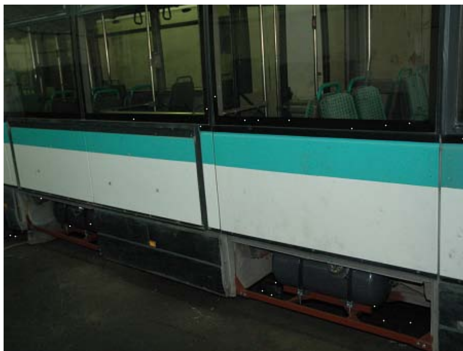
Fig. A5 LPG storage tanks mounted on the bus
