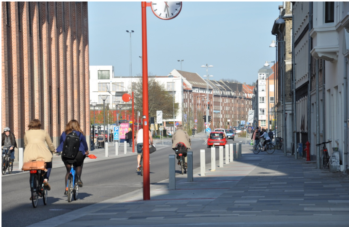
Figure 7: Narrow road profile to secure Shared Space use.
