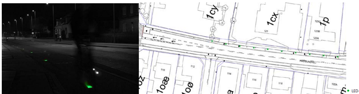
Figure 6: The placement of the 10 LED light at the Cycle motorway and the lights during night time.
