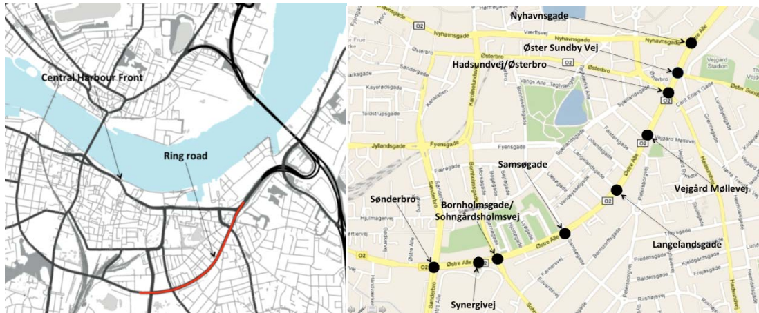
Figure 11 : Map with the included intersections in the Adaptive Traffic Signal Control System. Left: the location of the section of the ring road. Right: all equipped intersections. The intersections with Synergivej and with Bornholmsgade are together the double.
