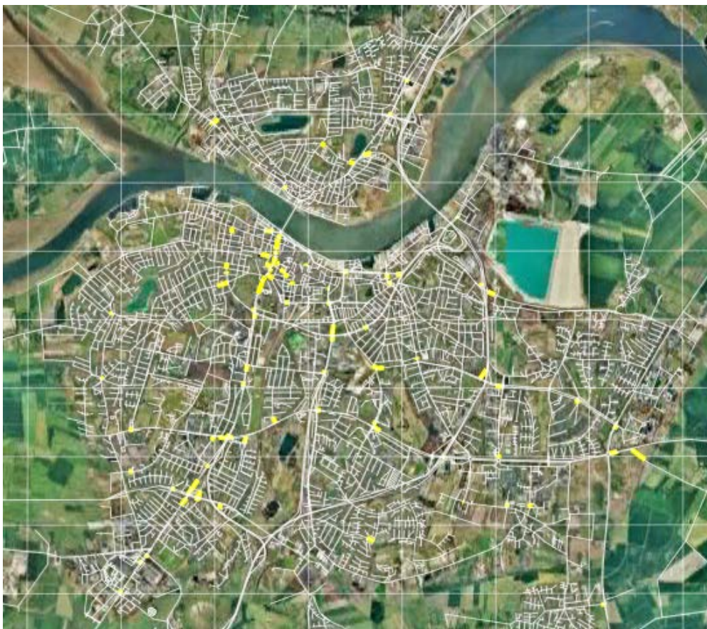
Figure 5 Bottleneck analyse showing bottlenecks where speed level drops to less than 50 % of free flow. Analyses from congestion monitoring system output on Google maps.
