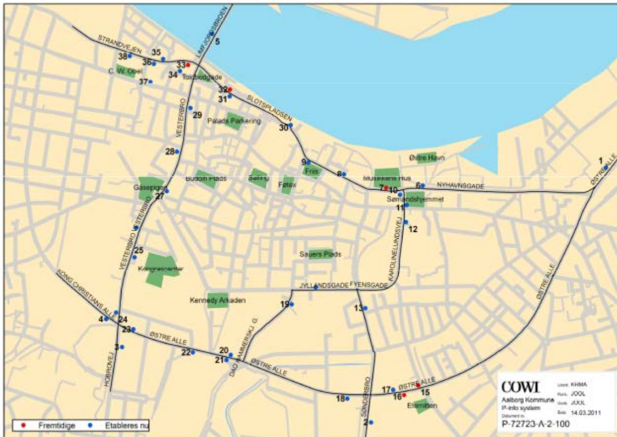
Figure 2: Map indicating the placement of the signs in the new Parking Information System. The green areas are present or future car parks. The blue dots are signs that will be established now, while the red dots marks planned signs to be established in the future
