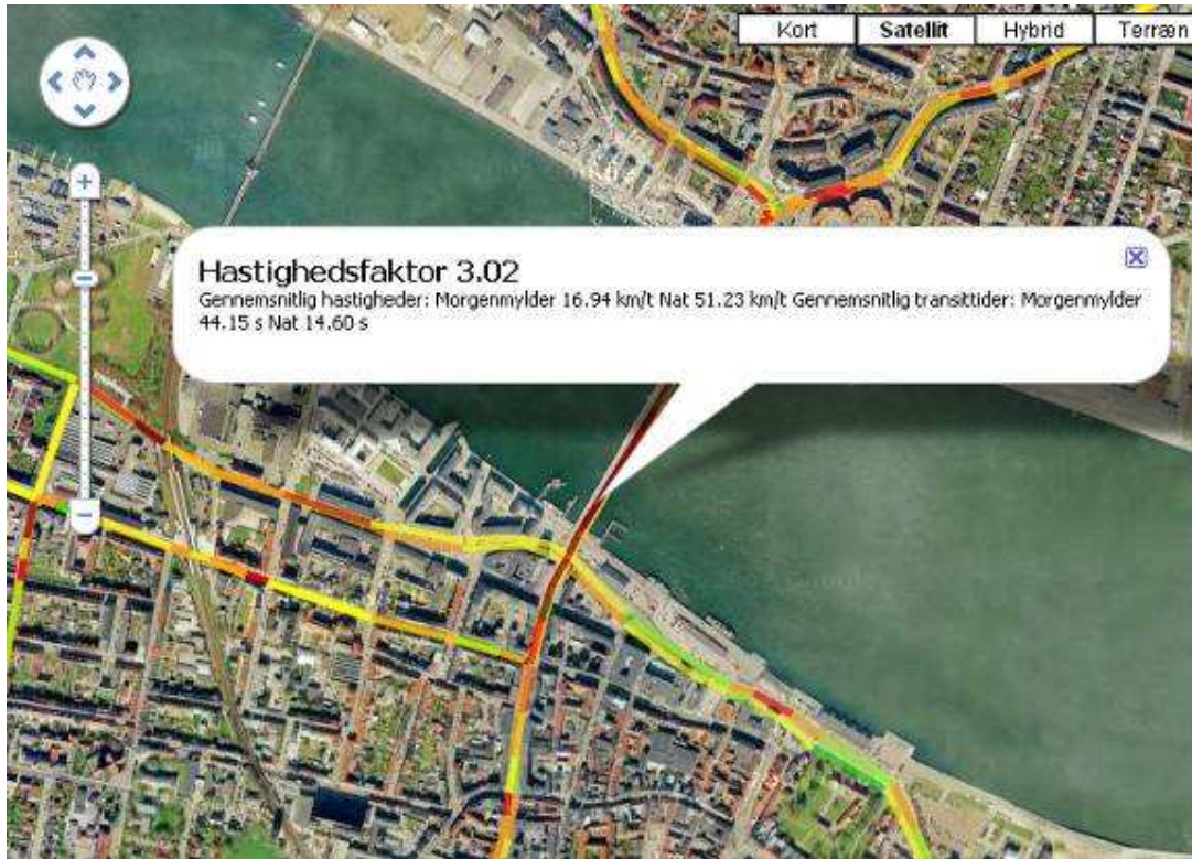
Figure 11 Road users can zoom in to see the speed profile or congestion level on each road segment in his commuter route. In this example, the label shows the congestion level as ratio between speed in morning peak hour (16.94 km/h) and in night free flow (51.23 km/h).
