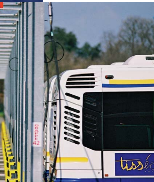
CNG Buses and filling station
