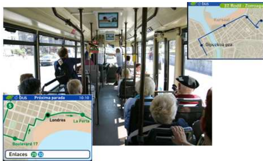
Figure 6: Onboard system information (DV-Bus channel) with next stop announcement
