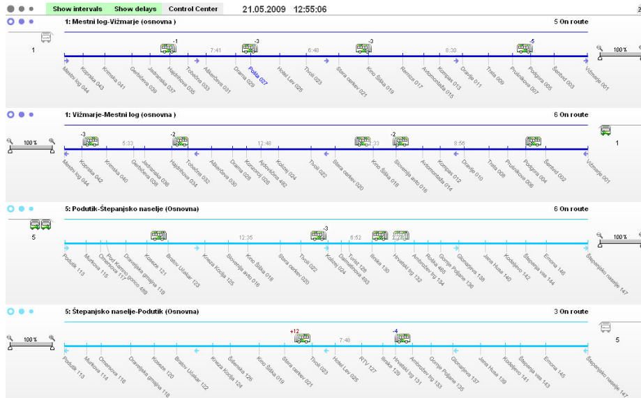
Figure 3: Routes (lines) with buses and bus stops presented on line diagram (real time information on vehicle's position)
