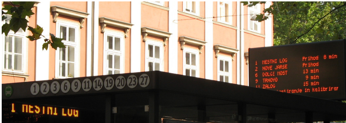
Figure 21: The objective of the project is also to implement direct communication technology for higher information accuracy – the system announces “prihod” (eng. arrived) when bus is at the bus stop
