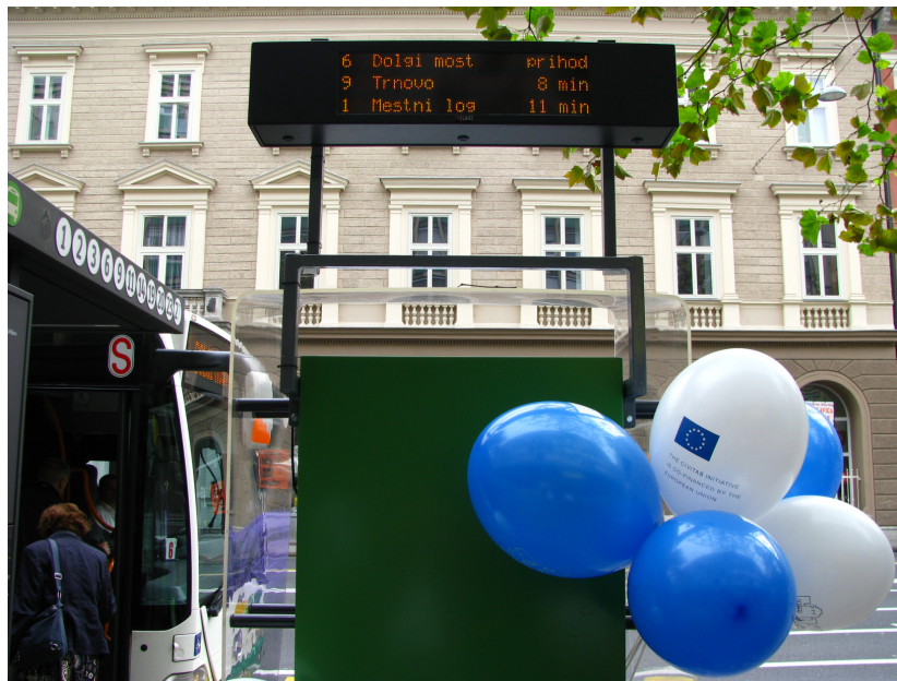
Figure 12: Part of the planning phase was also implementation of test electronic display at bus stop Konzorcij; however the test display didn't already include dedicated short range communication technology
