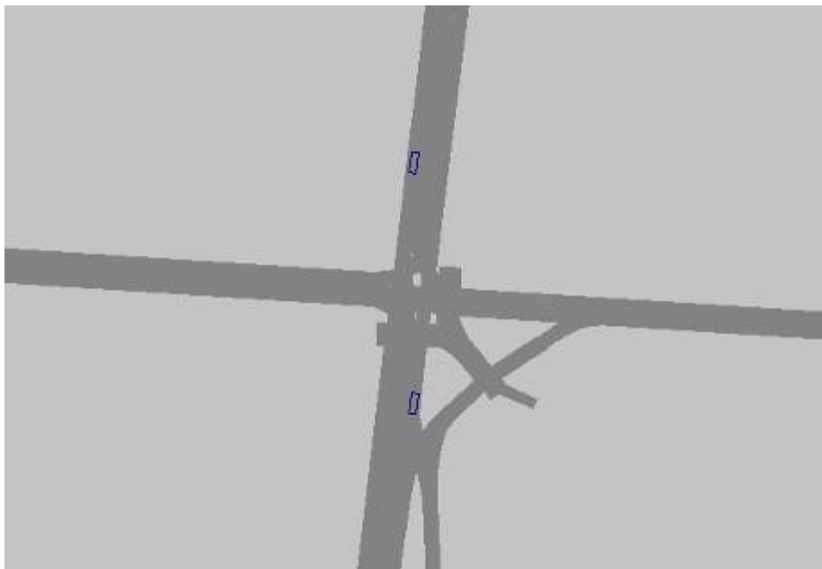
Figure 10: Detector placement in VISSIM simulation model
