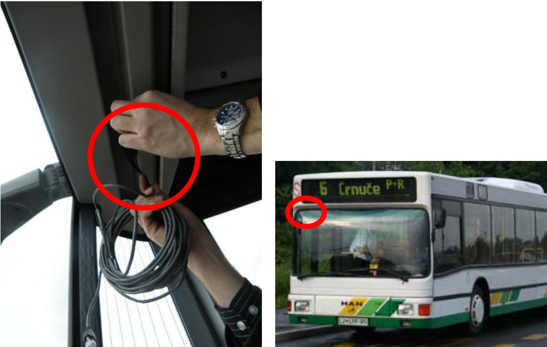
Figure 6: Location of Zigbee module in bus
