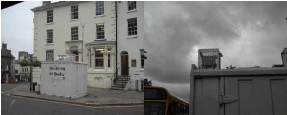
Testing the portable solid state NO x sensor unit on the mobile air quality station at the roadside in Castle Meadow.
