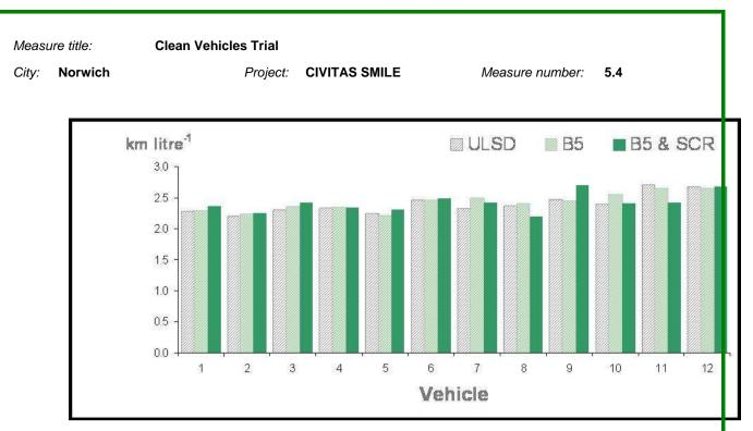
Fig 3. Fuel economy data for twelve First Bus vehicles running on ULSD, then on B5 and finally on B5 after retrofitting with SCR (selective catalytic reduction) to reduce exhaust emissions.
