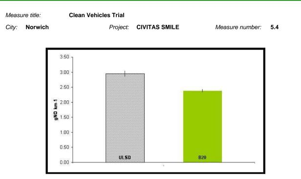
Fig 6. NO emissions per km measured on an Anglian Optare Solo Euro III bus (Mercedes 4.2 litre engine) using Autologic gas analysis equipment. Here we present the average of emissions integrated over a specified route for diesel (ULSD) and for B20 blend of ULSD with biodiesel. The error bars represent one standard deviation.
