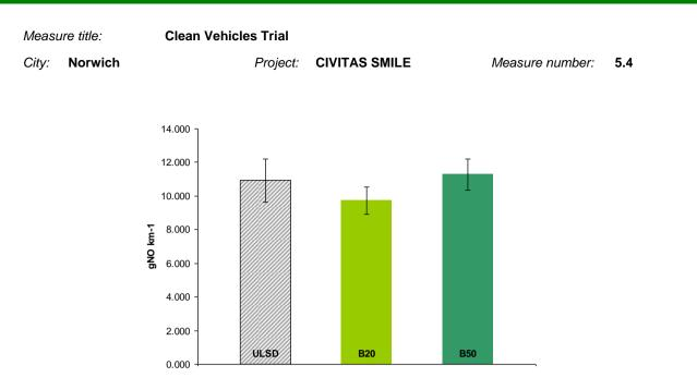
Fig 5. NO emissions per km measured on an Anglian Optare Solo Euro III bus (Mercedes 4.2 litre engine) with the exhaust fitted with Horiba gas analysis equipment to enable real-time monitoring of exhaust emissions. Here we present the average of emissions over particular parts of a specified route for diesel (ULSD) and for B20 and B50 blends of ULSD with biodiesel. The error bars represent one standard deviation.
