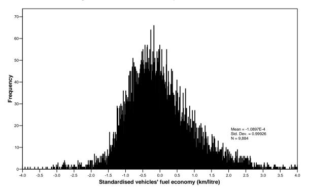
Fig 1. Raw Data taken from fuel economy records of 13 selected vehicles with nominally similar engines. The fuel economy data of each vehicle has been standardised and the data aggregated in the above frequency graph. Note the kurtosis of the distribution spread – the overall mean -1.069, biased by this distribution, is not a good measure of central tendency for comparative purposes.
