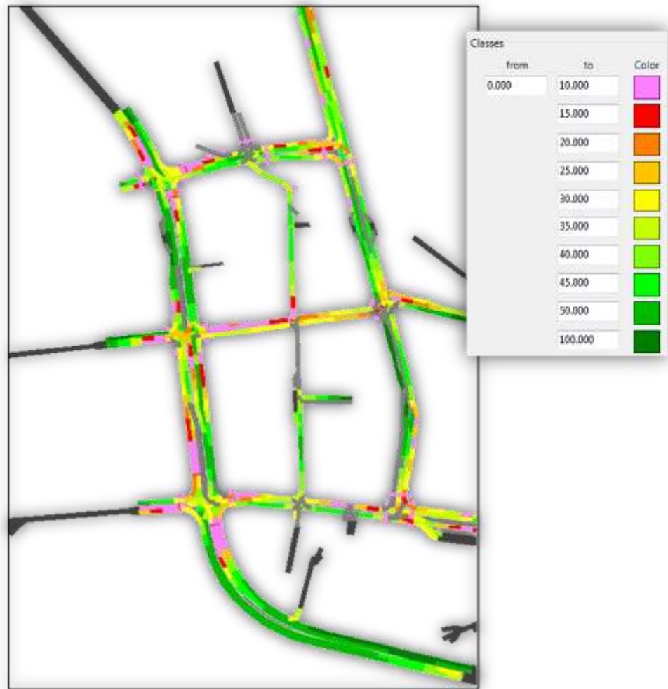
Figure 6 – Graphical representation of average driving speed in the area of the Masarykova street (year 2011, off-peak hour, all vehicles)
