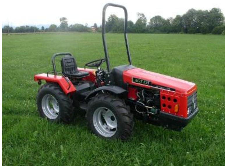
Figure 1: Tractor AGT 835 transformed to using pure plant oil, equipped with three cylinder water cooled diesel engine with direct injection of fuel, engine capacity of 1551 cm 3 , develops power of 26,4 kW.
