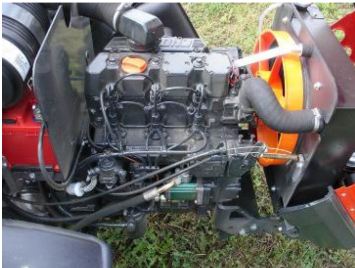
Figure 3: Original engine on tractor AGT 835 before conversion to pure plant oil
