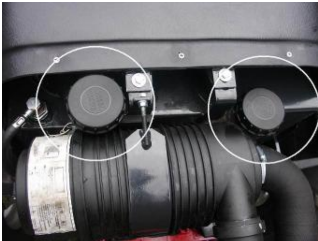
Figure 2: On the upper side of AGT 835 tractor engine two tanks are built in: the left smaller tank contains mineral diesel oil and the right larger tank contains plant oil
