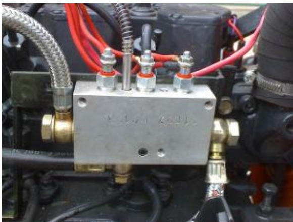
Figure 5: A detail of electric heater of fuel; in the heater the plant oil is heated to 80 – 95 °C so that the oil viscosity corresponds approximately that of mineral diesel oil
