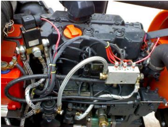
Figure 4: Engine on tractor AGT 835 after conversion to pure plant oil. On the left side of the engine is an electromagnetic valve which channels the fuel from mineral diesel tank or from pure plant oil tank; on the right side there is an electric heater which heats the plant oil to maximum value adjusted by electronic thermostat on the instrument board of the tractor
