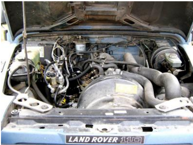
Figure 9: Conversion of engine on two tank system on vehicle Defender 110, Land Rover, on the left side of the engine is an electromagnetic valve which channels the fuel from mineral diesel tank or from pure plant oil tank to the electrical heating device for lowering viscosity of pure plant oil
