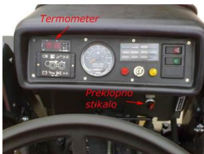
Figure 6: On the left side of control panel is electronic thermometer and on the right side is switch for selection of mineral diesel fuel use or pure plant oil use
