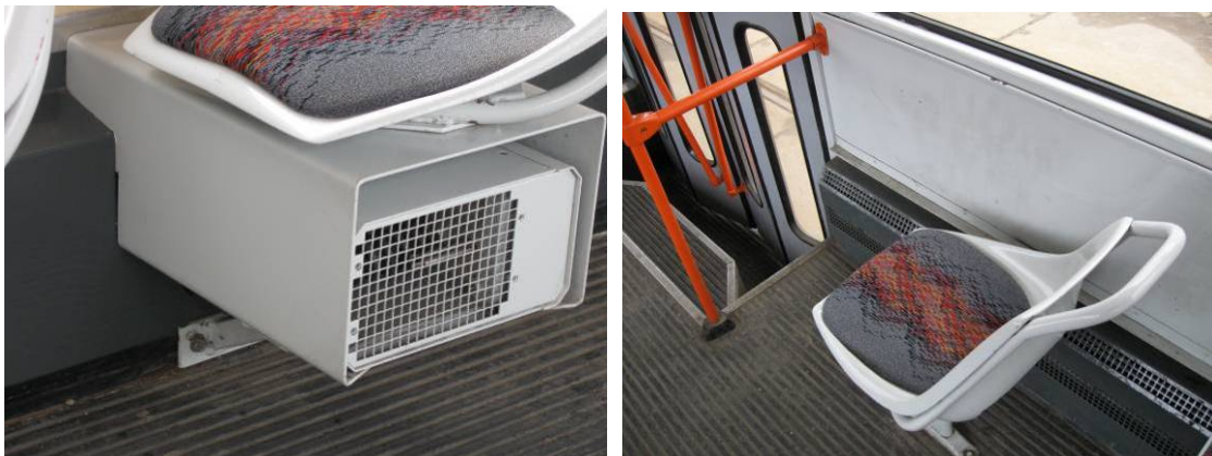
Picture 02: Heating system in trams and trolley-buses and its location
