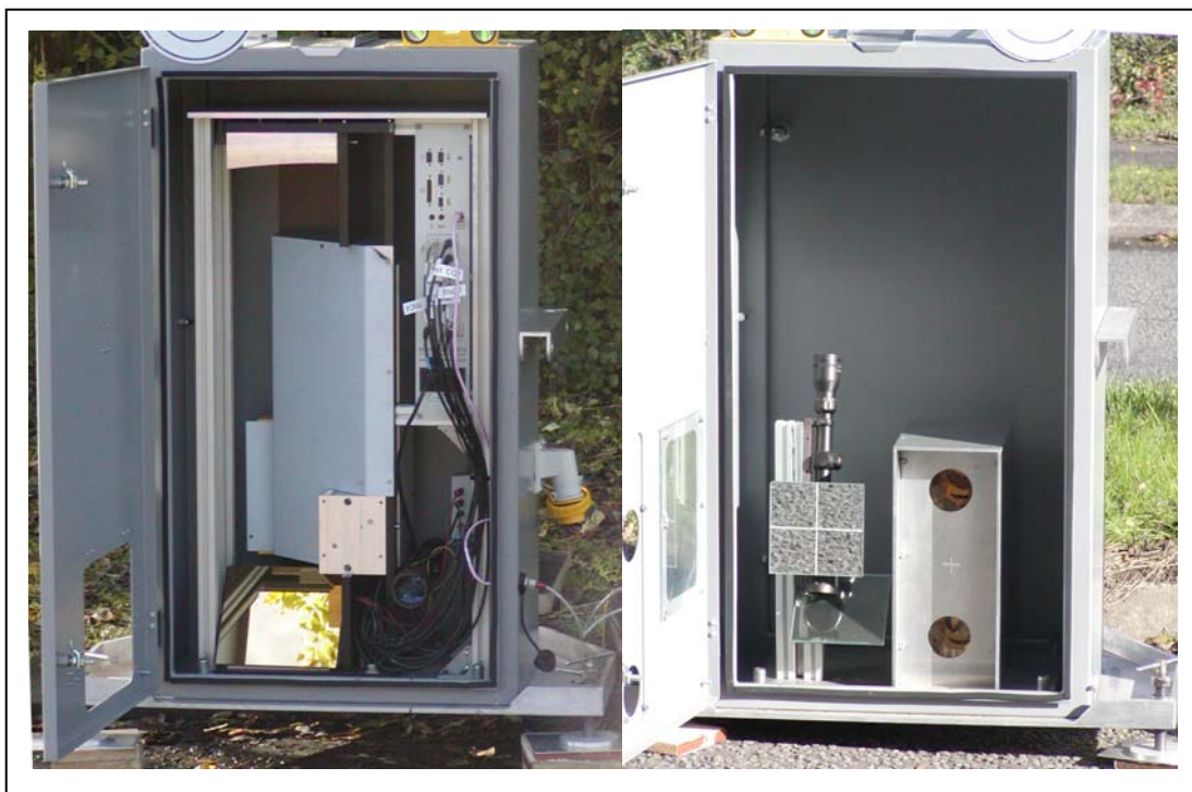
Figure 1: REVEAL RSD unit with i) main RSD unit ( left ) and ii) retroreflector unit ( right )
