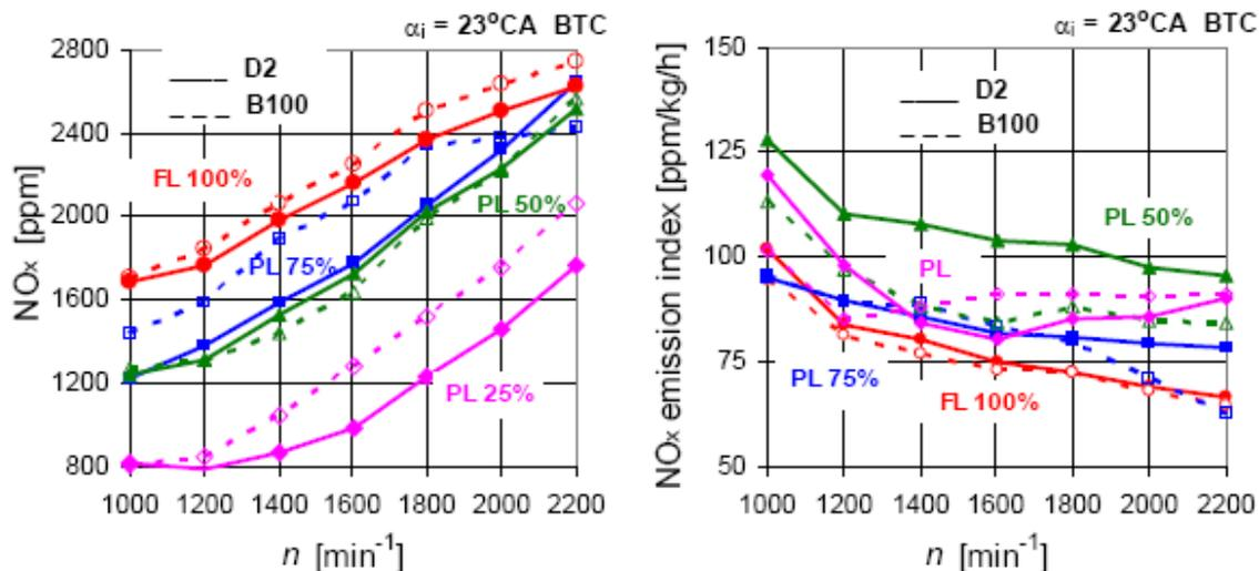
Figure 6: Emission concentrations and emission indices for NOx at different engine speeds on brake (rpm) and different loads (PL) using D2 or B100. Compared to other pollutants emission of NOx is the only higher for B100 than D2 – see also Figure 7 below.
