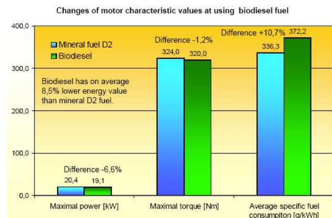
Figure 4: Tractor engine performance using D2 or B100
