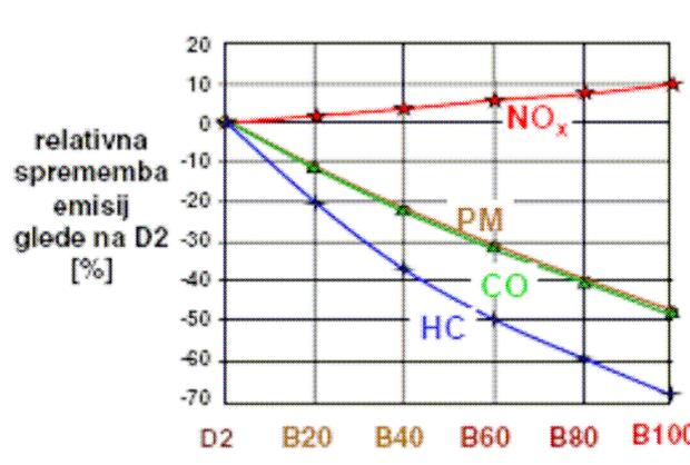
Figure 7: Relative change in emissions of HC, CO, NOx, and PM according to different B concentrations (B0=D2, B20, B40, B60, B80, B100=pure biodiesel). A reference is D2.
