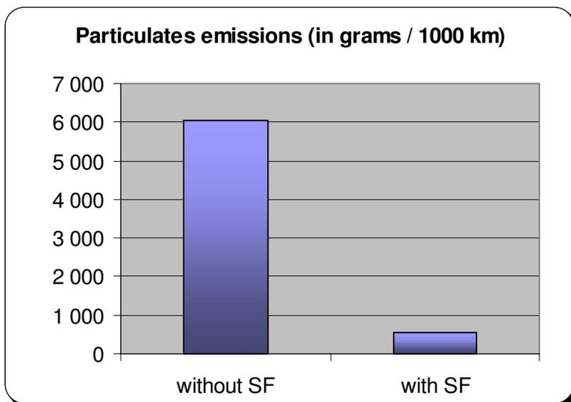
The buses fitted with particle filters emit much less particles than those that are not fitted with them (- 90.90%).
