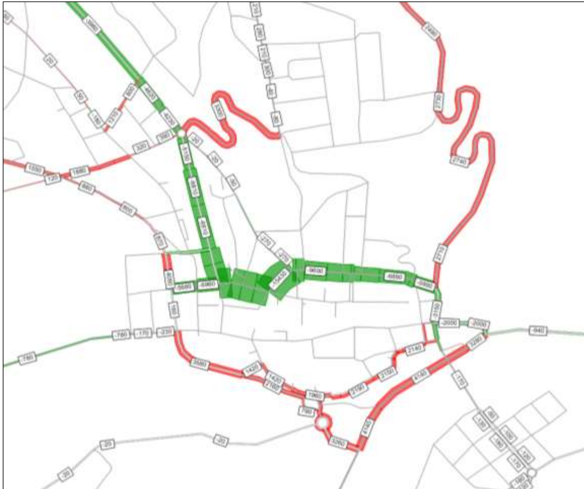
Figure C1.3.3: Changes of traffic intensities on roads in the city after measure implementation (green – decrease, red – increase of traffic intensity)
