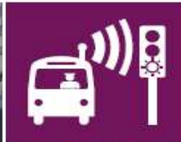
Priority at lights via radio. All intersections are equipped with a new system giving priority at traffic lights using a short-range radio.
